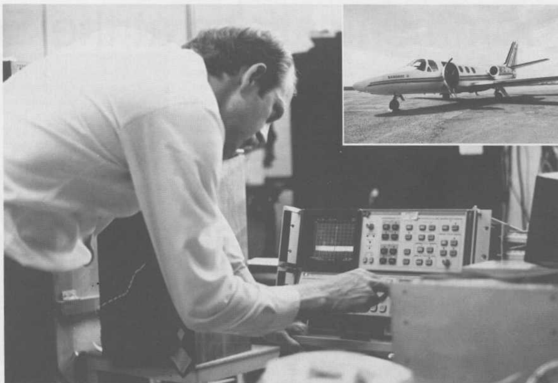
Mobile Satellite Systems Communications Engineer John Sydor conducts tests on the terminal which is used in Ontario air ambulances. The terminal is mounted in the "Bandage 4" (inset), one of several planes and helicopters paramedics fly to provide emergency medical treatment in remote locations.
