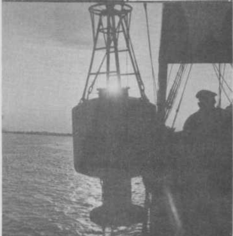
Buoy to mark navigation channel in St. Lawrence River being lowered over side of ship.
