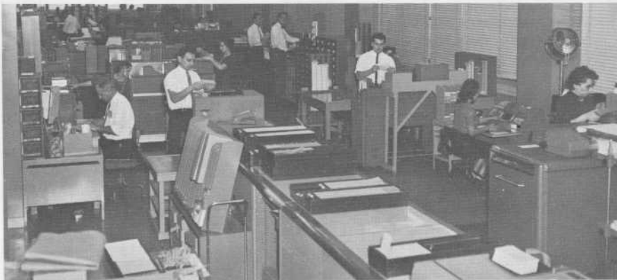
Thousands of weather reports from volunteers flow into the weather data processing section at meteorological headquarters each month. The information they contain is transferred to punched cards to give the vital weather data across Canada for any given month.
