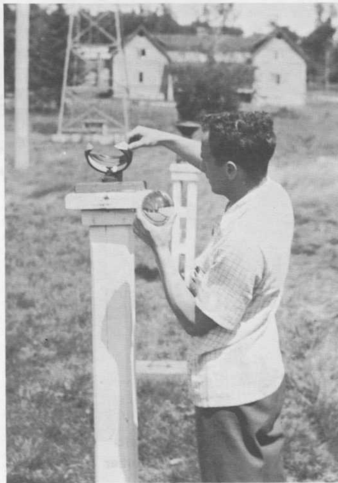
Two observers tend their daily chores, measuring rain (left) and changing sunshine recorder diagrams (right).
