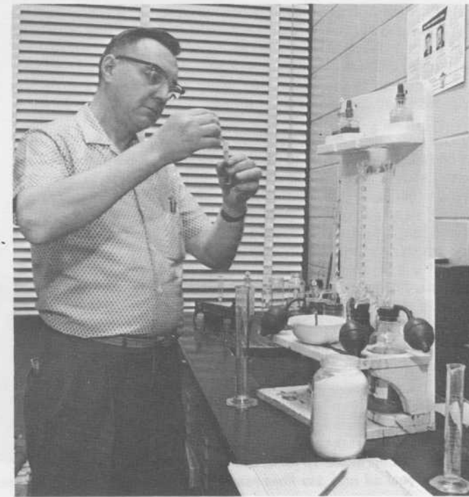
Bottom Right: Proper chemical concentration in high temperature and evaporator feed water is strictly controlled. Daily water test in plant lab is made by Shift Supervisor Morrow.
