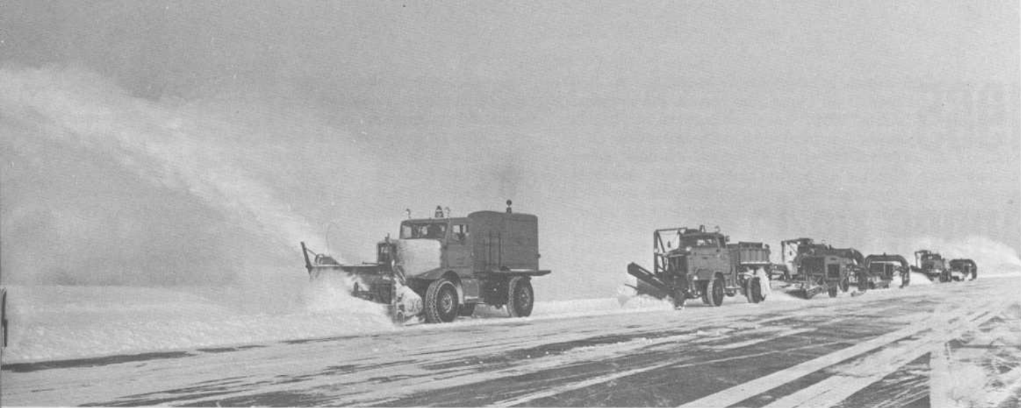
A convoy of plows and sweepers clean off Montreal's No. 24R runway, while aircraft land and take-off on a parallel one.
