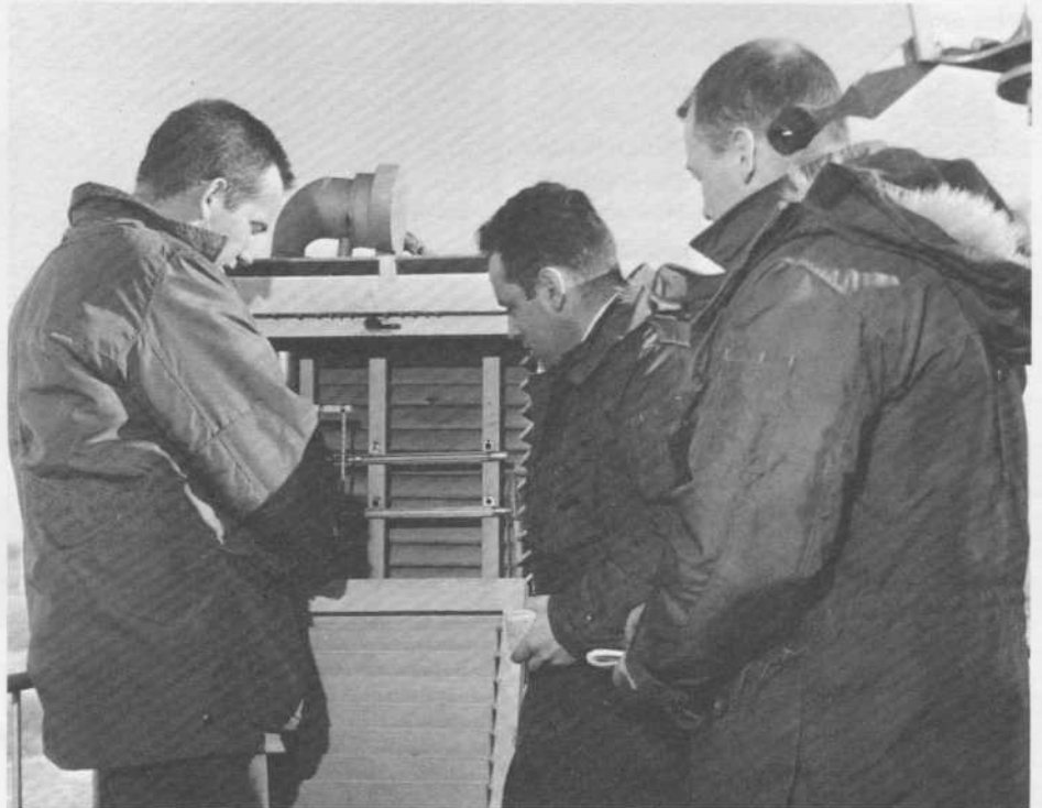
GATHERING THE BASIC INFORMATION— Instructor shows student met. technicians how to use the instruments in a Stevenson Screen at the D.O.T. Air Services School at Ottawa International Airport.
