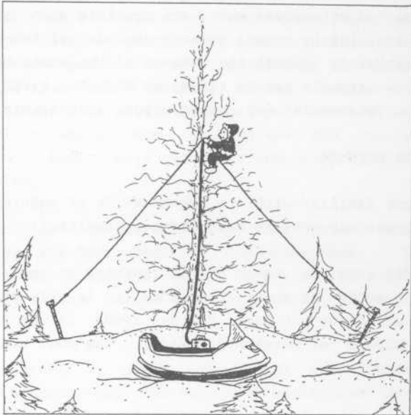
Figure 1: Ideally, the middle of the antenna should be 15 metres (50 feet) high and the ends 3 metres (10 feet) off the ground. Install your antenna as high as possible, avoiding obstructions which can cause interference.
