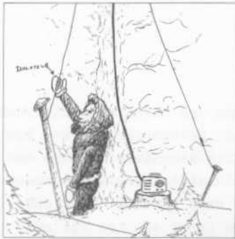
Figure 2: It is important that no radiating portion of the antenna come in contact with the ground.
