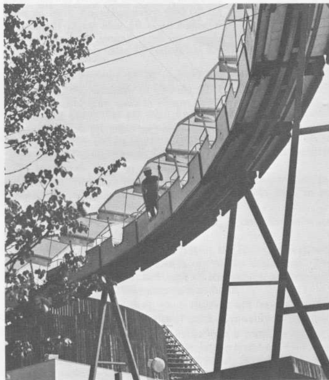
The Mini-rail will make up part of the secondary transportation system on the Expo 67 site. It's a single, elevated rail vehicle with open cars each carrying 12 persons. It is a mono-rail system in miniature.
